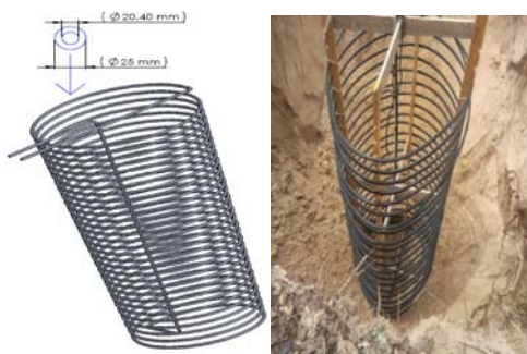
Fig. 2. Dimension and Schematic diagram of the CBGHE
